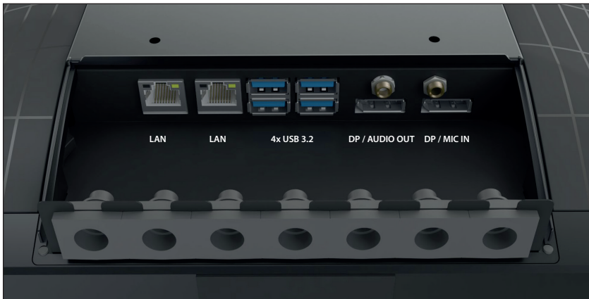
Figure 7.3 Connectors of Uniq PC 150 II Celeron 4305UE / Core i3-8145UE
